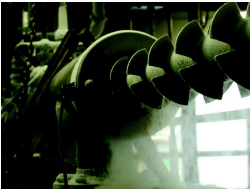
Opened screw conveyer for material cooling with liquid nitrogen
