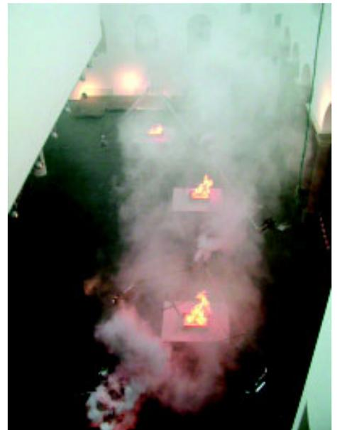
Practical smoke test in an atrium building: smoke layer below the ceiling
