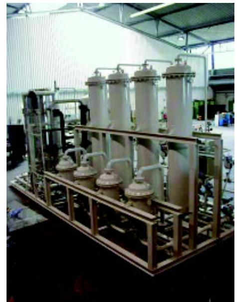
Pressure swing adsorption plant
