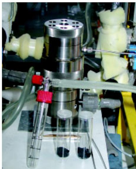
Detail view of the system used for high pressure impregnation of activated carbon
